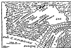
FIGURE 118—The structure of Lake Superior showing the fault blocks (Horst and Graben) which help to build it. (Partly after F. B. Loomis) (Atitokan should be Atikokan)
